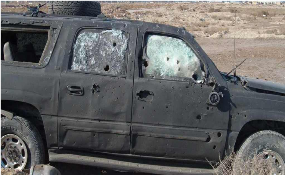
Picture 8 – Armoured vehicle damaged by "EFP"
